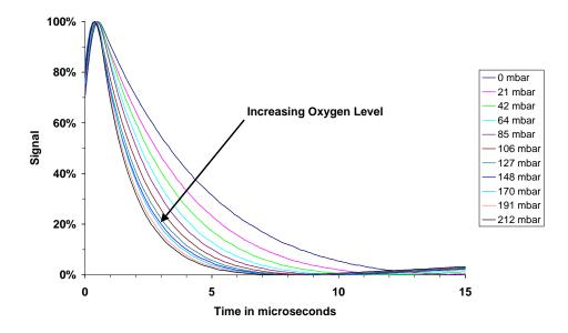
Fluorescence decay curves for differing concentrations of oxygen
