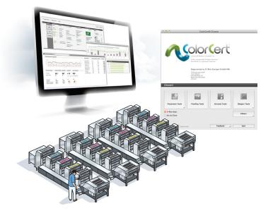
spectrophotometric devices. The end result is the reduction in variances among measurement devices caused by age, wear or environment. Investing a few minutes each month in certifying the accuracy of instruments reduces rework, speeds time to market, improves quality and repeatability and has a direct impact on profits.
