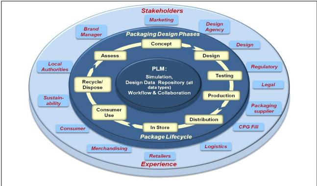
Figure 4: Concurrent packaging design rests on having technology to simulate the package at all phases, store information from all elements, and allow stakeholders to collaborate at any time.
