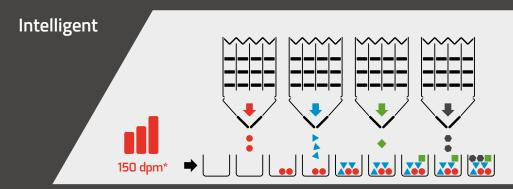
A typical 'Intelligent' model has three memory flap units and is best suited for counting small product quanties (1-10 product per pack) at very high speed.
