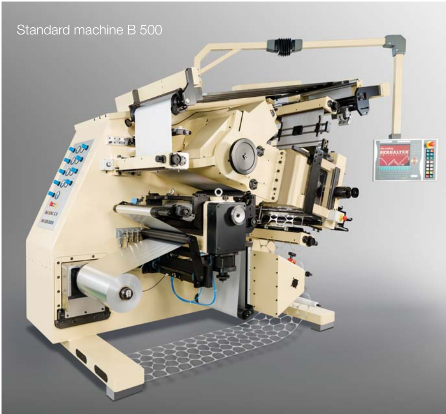
Machine B 500 with REELsplicer™, PRINTinspect™, WEBinspect™, WEBslitter™ and BEAMstack™
