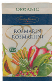
Aroma barrier paper sachet Paper//PE/tie/EVAL™/tie/PE outside inside
