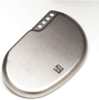
A pacemaker has been permanently marked with a Data Matrix symbol using a method of direct part marking (DPM) called laser etch.
