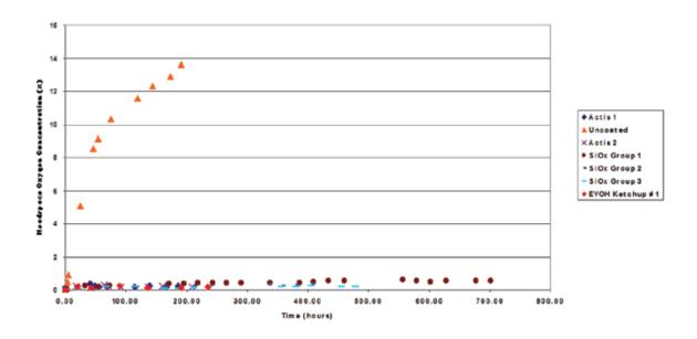
Oxygen permeation into PET bottles with different oxygen barriers (dissolved in liquid) measured over 700 hours
