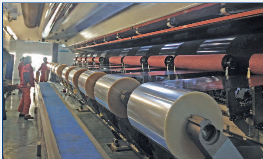
10.4m wide Atlas CW1040 primary film slitter during commissioning at Jiangsu Hengchuang Packaging Material Co. Ltd.
