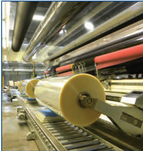
The recently commissioned Atlas CW1040 primary film splitter in action at Uniscite, Inc.
