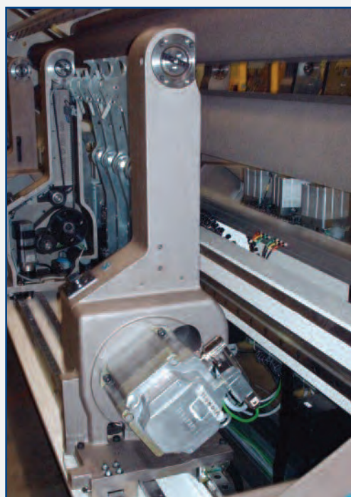
All 14 obsolete motors were replaced on the rewind arms with Siemens AC servo motors
