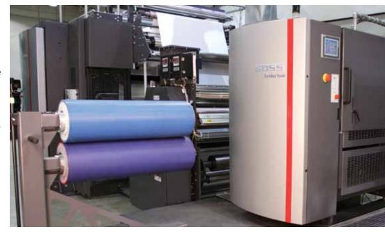
20 years of sleeve press experience allowed Goss engineers to quickly perfect the air pressure and cylinder registration mechanisms for fast, simple size changes.
