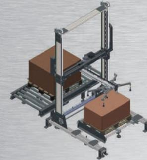
The pad-inserting module is a pad feeding system adjustable in accordance with the size of the interlayer pad, that can be combined with the central column of the APS ERGON palletizer. Suction-cup gripping system from 4 up to 8 adjustable points to ensure the accurate lifting of any kind of interlayer. The interlayer pad automatic loading is available as optional and allows to load the pallet
