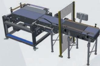
Single-entry infeed with 90° layer-forming system equipped with: 1 rubberized cadencing belt, 1 product infeed belt, in order to form the row and 1 one-way translation system that contributes to forming the layer into the basket. The layer-forming system is
