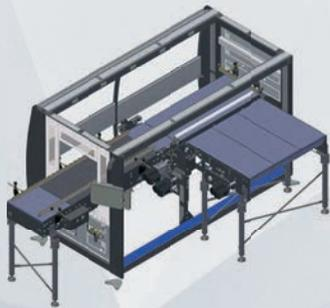
Single-entry infeed with 90° layer-forming system equipped with: 1 rubberized cadencing belt, 1 product infeed belt, in order to form the row and 1 one-way translation system that contributes to forming the layer into the basket. The layer-forming system is equipped with energy-efficient motors. Designed in
