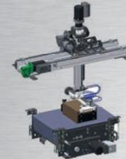
On the APS 1570 pack rotation can also be carried out by a motorized manipulator (optional device).
