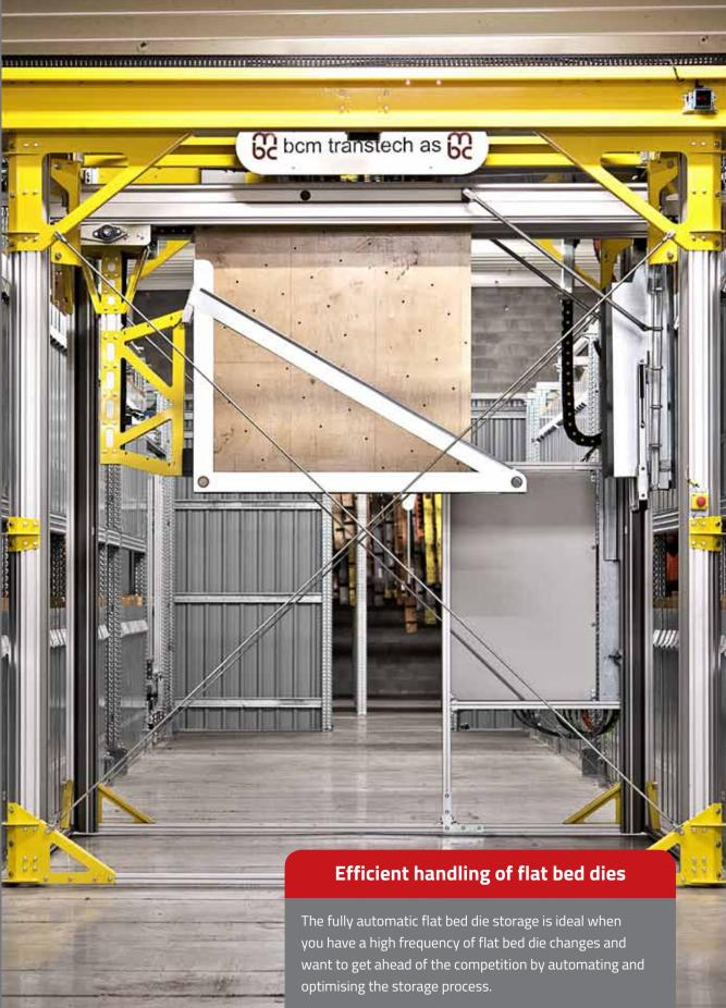
Specifically, it lets you run a high-volume storage with few operators, because the storage unloads and loads the transport trolleys, while the operators can solve other tasks. In addition, the storage keeps track of the flat bed dies, so that it is easy to locate them.
