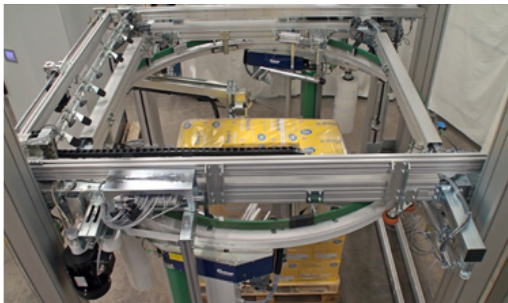
This is the GL 2000 Twin in action, wrapping a pallet of goods. Note the twin devices which encircle the pallet.
