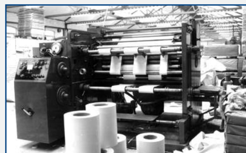
The Titan SR2 slitter rewriter (circa. 1965) many of which are still in production today
