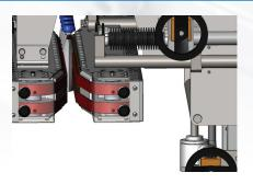
Fine tune adjustment for precision pressure sensor position.
