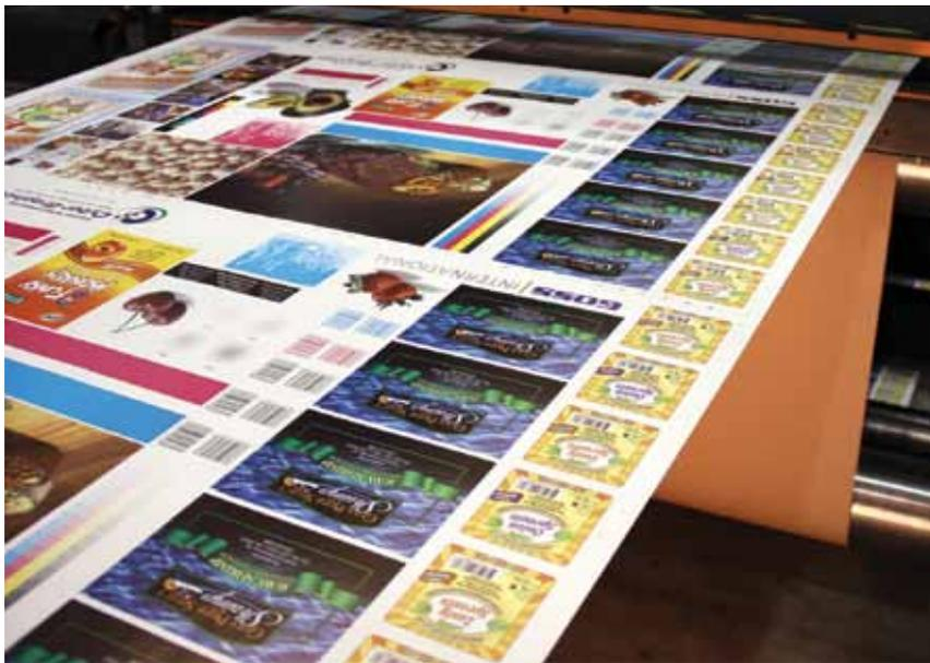
*The Goss Sunday Vpak packaging press – here outputting to 18pt SUS paperboard – is available in web widths up to 1905mm*
