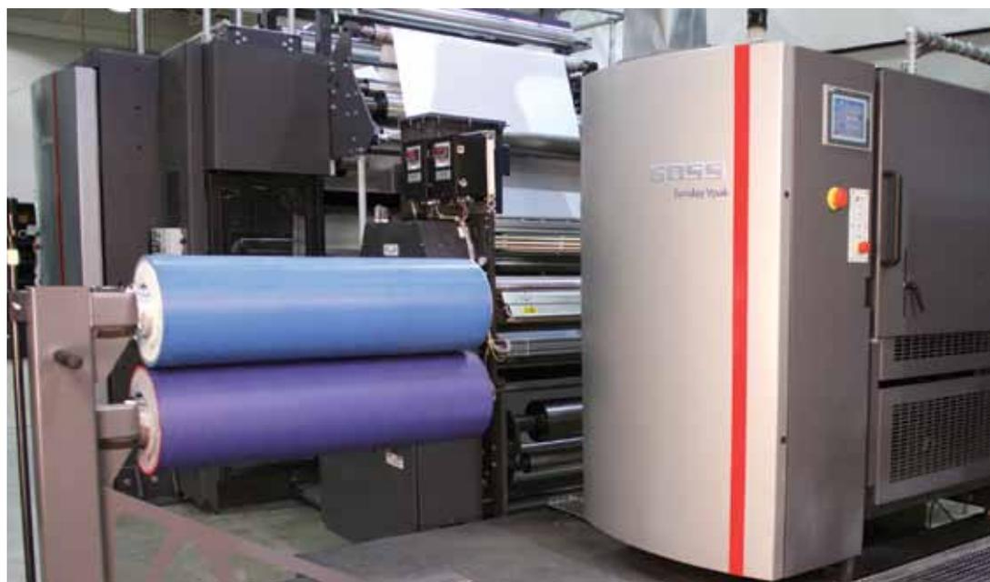
*20 years of sleeve press experience allowed Goss engineers to quickly perfect the air pressure and cylinder registration mechanisms for fast, simple size changes.*
